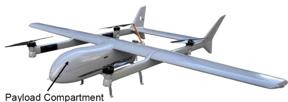
Fig. 4. Drone type assumed in this study. The drone is an electric VTOL/FW hybrid (5 m wingspan). Cargo bay is sufficient to accommodate one medium-sized medical container. Source: adapted from Mugin [59].
